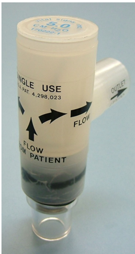
Fig. 1 Photograph of the bronchospasm device model. One port at the bottom (port A) of this picture is attached to the lung simulator (i.e., the patient), while another port on the side (port B) is connected to the ventilator in this experiment
